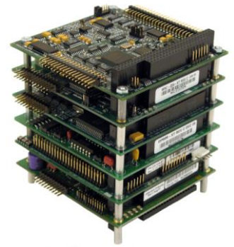
Figure 1 Older design consisting of cumbersome stacks of SBC and I/O modules
