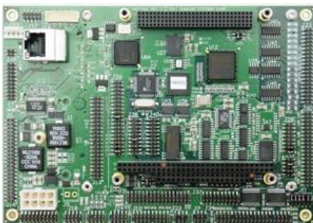
Figure 3 Neptune's I/O rich baseboard replaces the stack of modules in Figure 1
